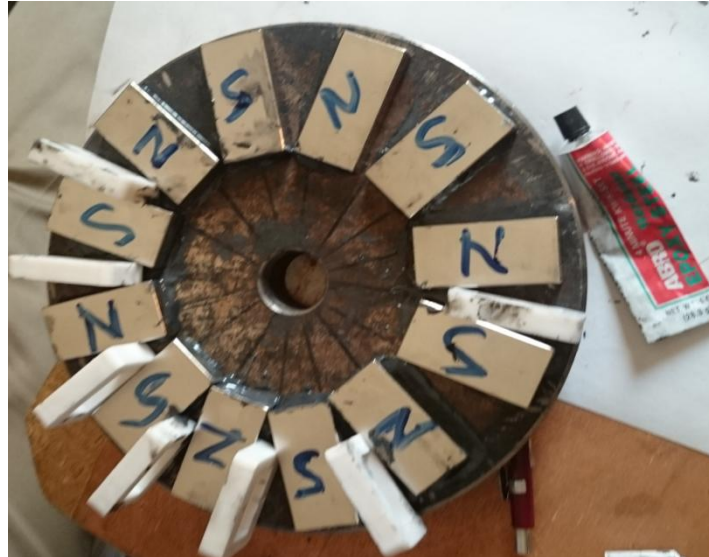
Fig5: Magnets mounted with poles opposing each other
