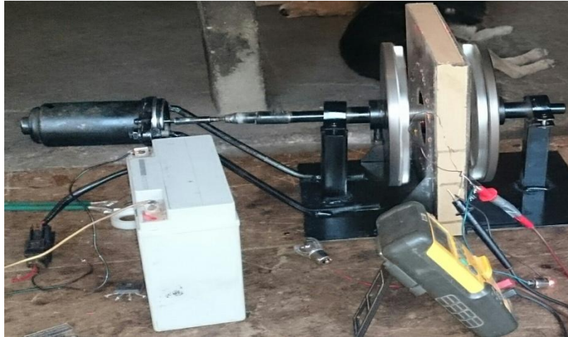
Fig8: The assembly of the wind turbine generator with tachometer to measure speed
