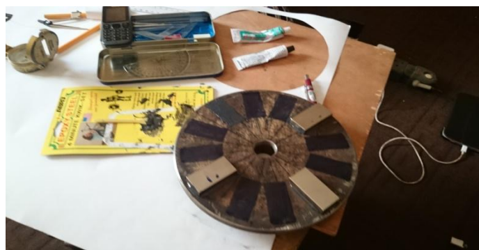
Fig4: Progressive mounting of the magnets
